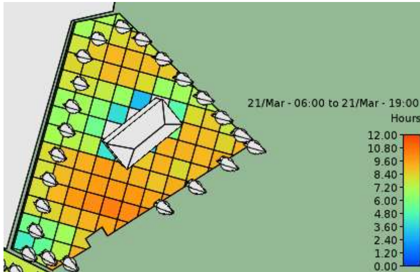
Figure 38: Sunlight hours to Existing Dwelling F on March 21 st more than 50% > 2 hours (Source IES VE SunCast)
